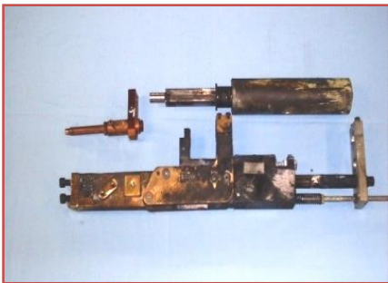
Weld Gun AFTER Rebuild
